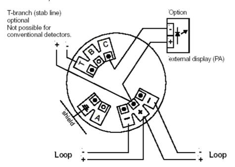
Binder A and B are for free disposal For conventional detectors a terminator must be set 5k6 in the last detector.
